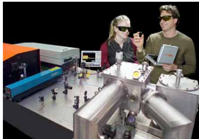
Atom optics experiment for focusing neutral helium atoms. ( www.physics.monash.edu.au/staff/research/bishop.html )
